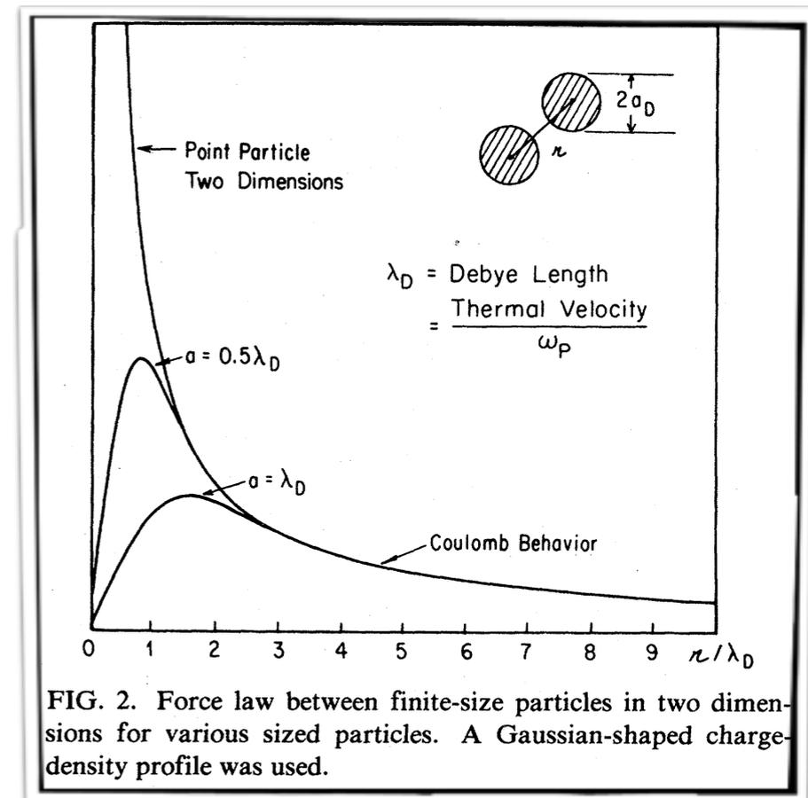
FIG. 2. Force law between finite-size particles in two dimensions for various sized particles. A Gaussian-shaped charge-density profile was used.
