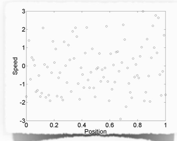
Particle distribution function represented by **macro**particles on a numerical grid.
