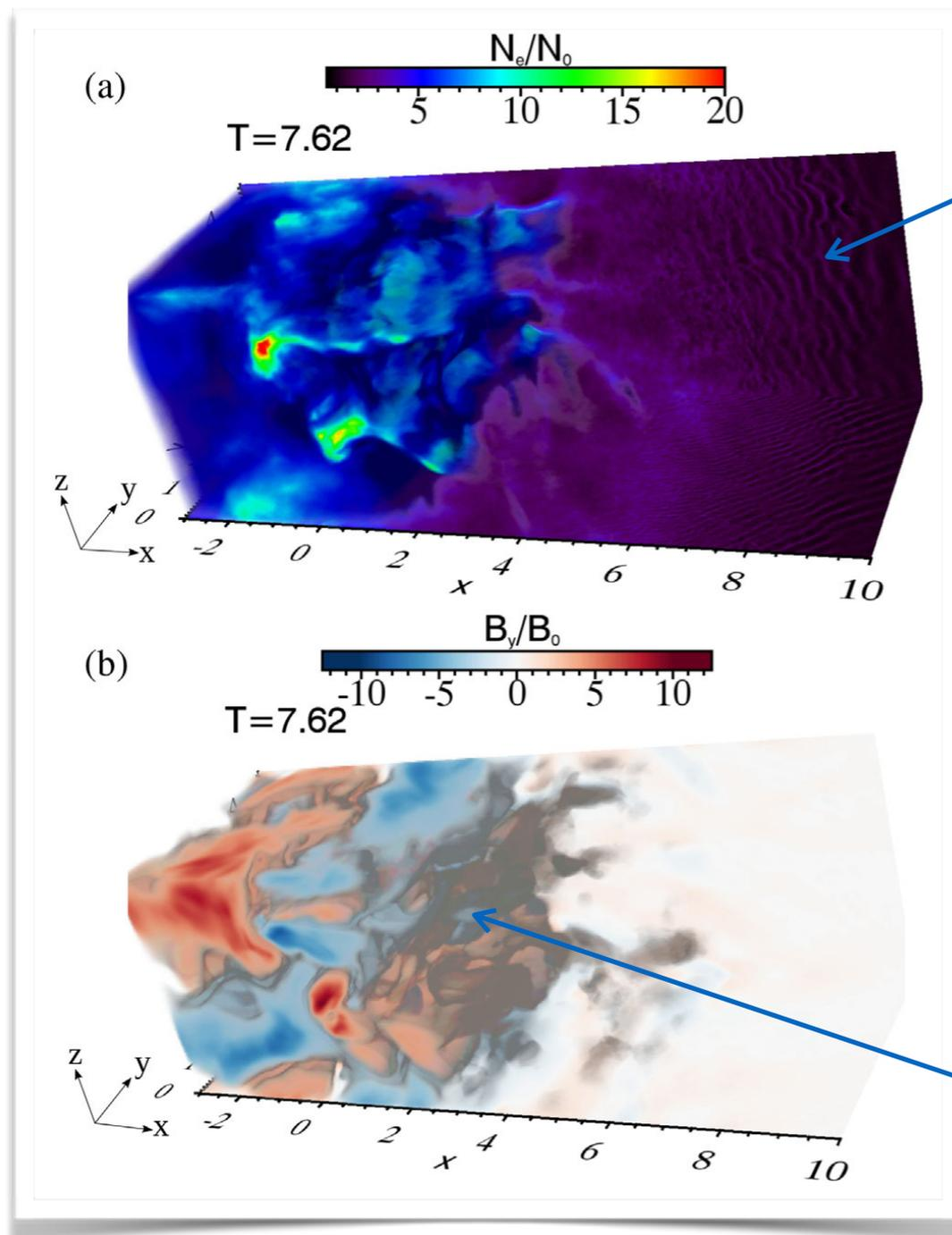
*coherent electrostatic structures in the shock foot ( $|E| > B_0$ )*
