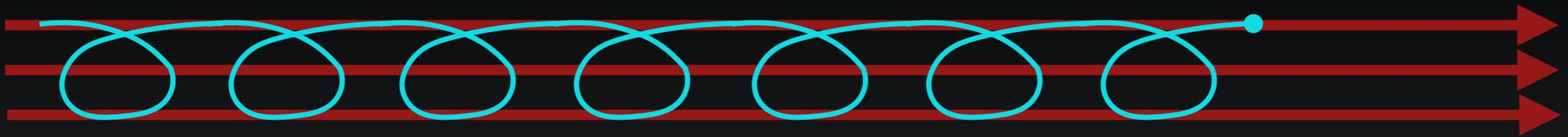
$$\rho \frac{d^2 \mathbf{s}}{dt^2} \sim -\frac{1}{c} \mathbf{j}_{\text{cr}} \times \mathbf{B} \quad \Rightarrow \quad \Delta s \sim \frac{j_{\text{cr}} B}{\rho c} t^2$$
